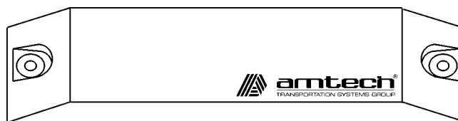
Figure 2-17 Transportation Tag Mounted with Rivets
