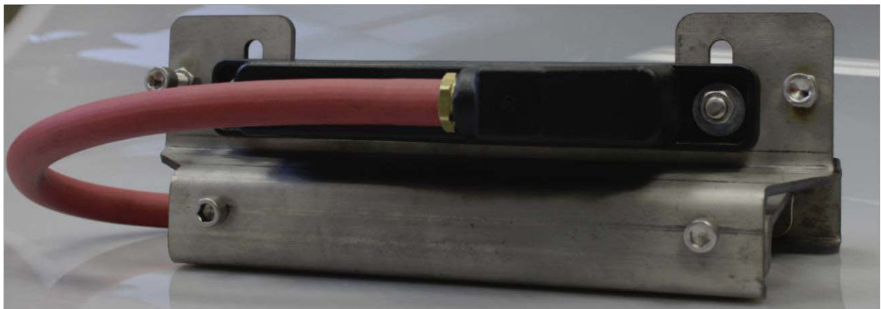
Figure 5 Sensor on bracket with the correct, right-side up orientation
