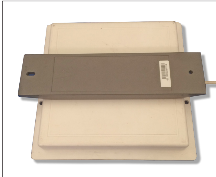
Figure 29 Tag and Antenna Orientation (horizontal polarization)
